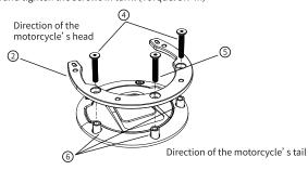
3. Place part ① on top of part ② (note to align the holes), put in the screws, and tighten the screws in turn. (Torque: 1.5N·m)
