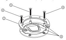
3. Place part ① on top of part ② (note to align the holes), put in the screws, and tighten the screws in turn. (Torque: 1.5N·m)
